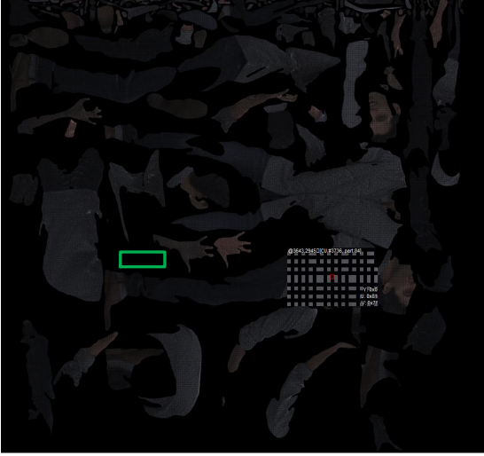
Fig. 4. Typical example of a projected view with the unoccupied pixels set as black from the plenoptic point cloud ‘‘Loot’’.
