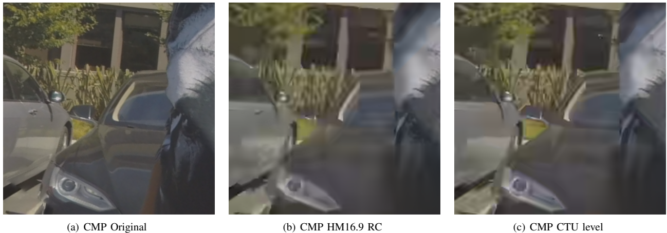
Fig. 5. View port subjective improvement of the CMP format. Test sequence: SkateboardInLot. Picture order count: 16. The region shown is a cropped 400 \times 400 zone starting at (500, 800) from the view port (75, 75, 0, 0) with size 1816 \times 1816 . (a) original sequence; (b) HM16.9 RC (bitrate: 2021.3kbps); (c) HM16.9 CTU level (bitrate: 2020.9kbps).
